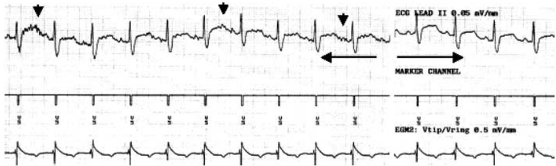
Figure 1. The programmer electrocardiogram (top trace) of one ICD recipient (Patient 40) showed artifacts (indicated by arrows) while the one mobile phone was ringing, and while the investigators were communicating over the two phones (8594;). The simultaneous intracardiac electrocardiogram revealed no artifacts. The artifacts disappeared when the mobile phones were switched off (8594;).
