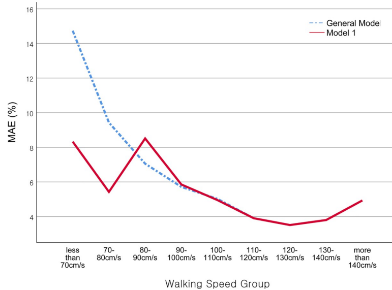
Fig 3. Accuracy of walking speed estimation algorithm according to reference walking-speed group. The general model (indicated by the dotted line) exhibits an inverted j-shaped curve. The MAE increases gradually at low walking speeds. However, the algorithm applying the low-speed-specific model (M1, indicated by the solid lines) limits the MAE increase at low walking speeds within a certain range. (Note. MAE, Mean Absolute Error).
