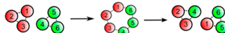
Figure 4. Circles 1–3 and 4–6 show two aggregates consisting of stickers which change their composition via cluster association–dissociation processes. This process leads to a partner exchange event which is followed by stress relaxation. Adapted with permission from ref 47.
