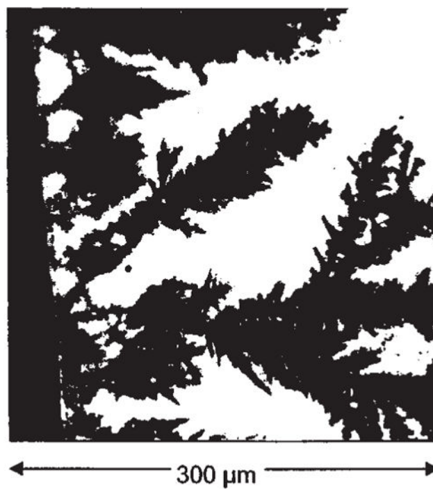
Fig. 4. Top: configuration for creation of fractal silver surfaces on silver electrodes and glass. Bottom: silver structures on or near the silver cathode. Bright field image.
