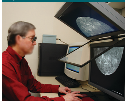
Figure 7: Stereo display workstation for mammography. This dual-display system based on a prototype high-resolution display (StereoMirror; Planar, Beaverton, Ore), utilizes passive cross-polarized glasses.
