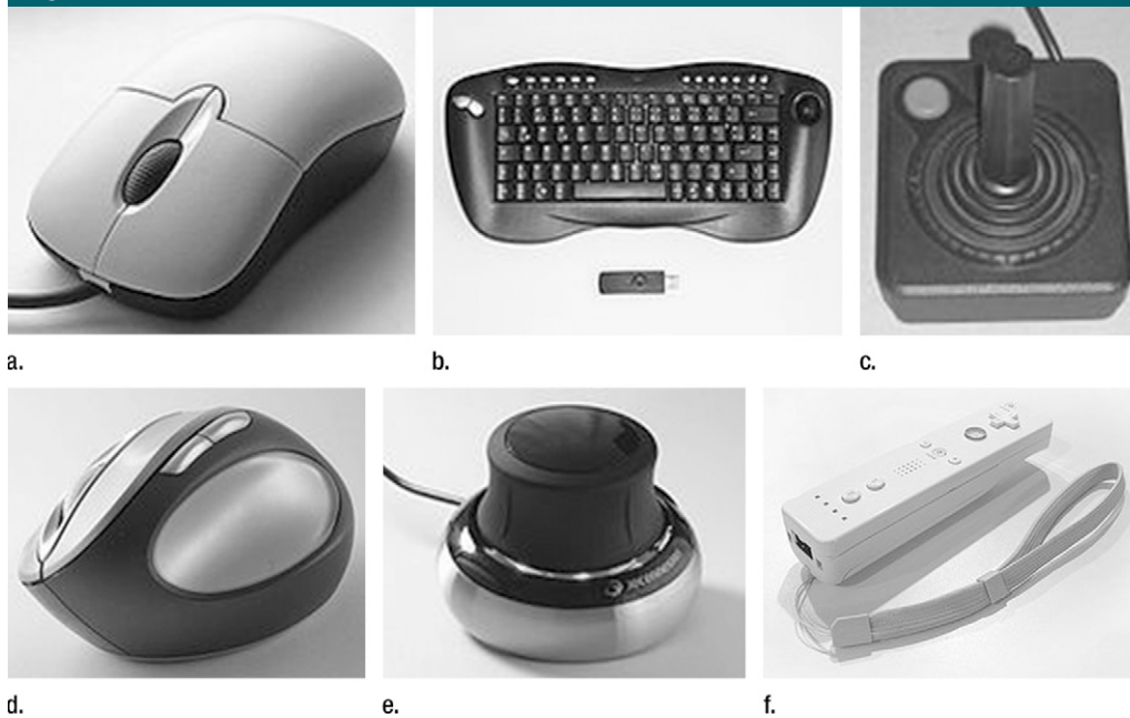
Figure 13: Composite historical array of computer interface devices from the public domain. (a) Computer mouse with standard features of two buttons and a scroll wheel. (b) Wireless keyboard with trackball. (c) Joystick. (d) Advanced five-button mouse. (e) Three-dimensional motion controller navigation device with six degrees of freedom commonly used in 3D modeling and animation. (f) Gaming controller that utilizes motion-sensing optical technology.
