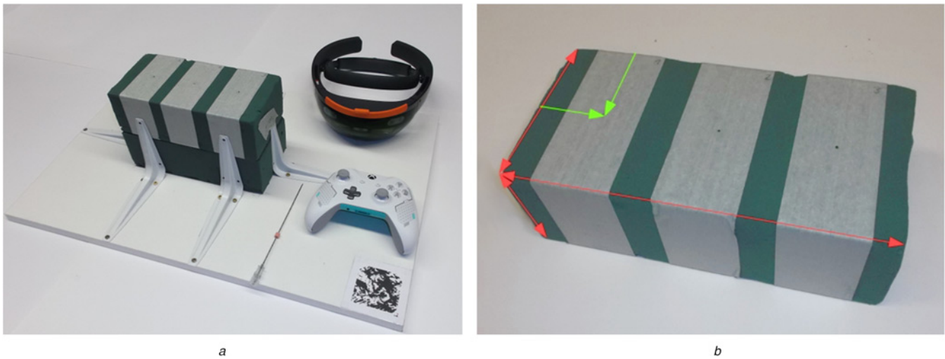
Fig. 4 Apparatus used for comparison study a Registration board, floral foam bricks, needle applicator, HoloLens and control pad b Measured distances at a floral foam brick
