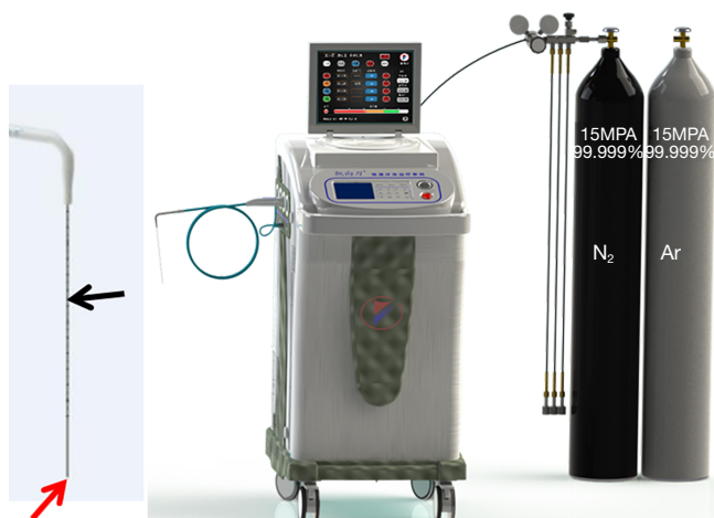
Figure 1 The cryoablation device (AT-2008-II, AccuTarget MediPharma, Shanghai, China). The working pressure is 8,268–10,335 kPa (1,200–1,500 psi) with argon and Nitrogen as the refrigerant, and it has 4 independent output channels. The length of cryoprobes (black arrow) and the diameter of the cutter head (red arrow) are 17.5 and 0.15 cm, respectively. The length of the frozen area is 3 cm.
