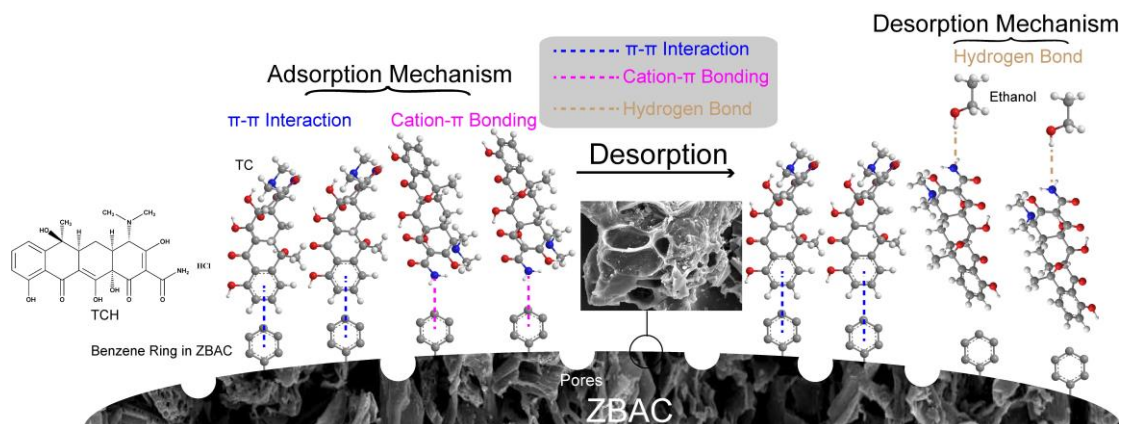
Figure 9. The schematic diagram illustrated the TCH adsorption and desorption mechanism on ZBAC.
