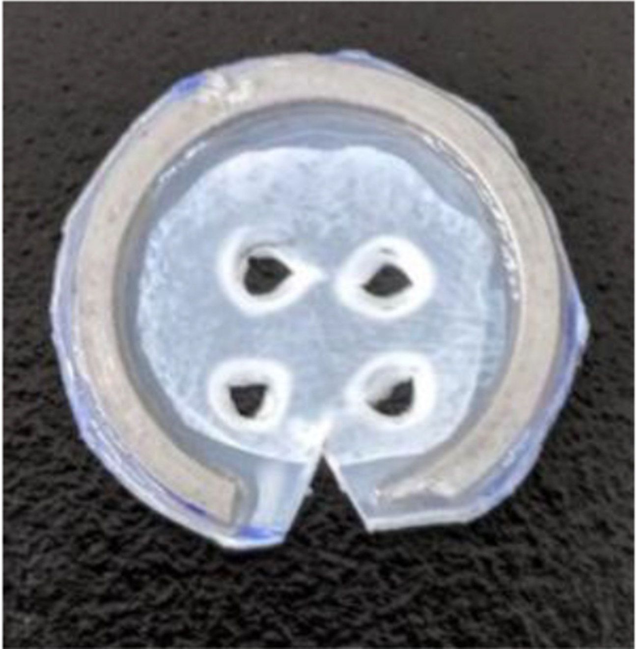
Fig. 8. ABS plastic film disk used in LCNIS haptic cartridge. Four distinct puncture holes are shown from four insertions using the LCNIS.
