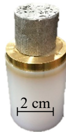
Figure 2. Closed-cell foam specimen mounted on projectile.
