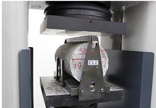
Figure 5. Setup of indirect tensile test.
