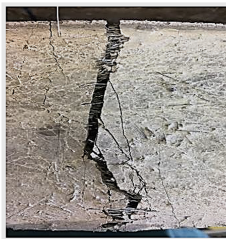
(c) Flexural test: Steel Fiber Reinforced Concrete (SFRC) (left); and Engineered Cementitious Composite (ECC) (right)
