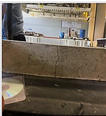
(c) Flexural test: Steel Fiber Reinforced Concrete (SFRC) (left); and Engineered Cementitious Composite (ECC) (right)
