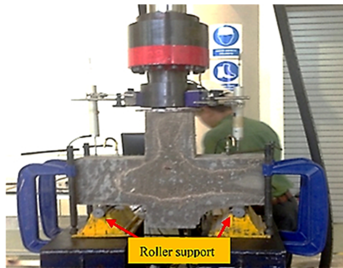
Figure 3. Setup for three-point bending test.
