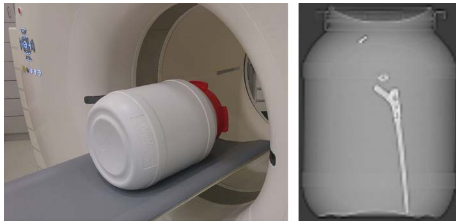
Figure 1. Phantom construction containing standard hip implant and a solution of ^{18}\text{F} -FDG and water. The phantom simulates a pelvis in a PET/CT scanner (left image), where the hip implant is lying freely in the phantom (CT topogram, right image).
