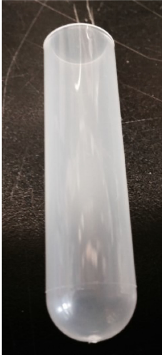
Figure 2. Beckman ultracentrifuge tubes. Ultracentrifugation tubes utilized to pellet vesicles.
