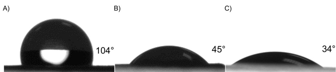
Figure 4. Water contact angle of PCL-ref (A), PCL-COOH (B) and PCL-TiCaPCON (C).
