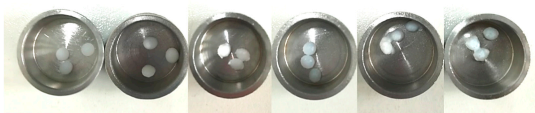
unprocessed PCL 2 h adsorption 4 h adsorption 6 h adsorption 15 h adsorption 24 h adsorption (a) (b) (c) (d) (e) (f)
