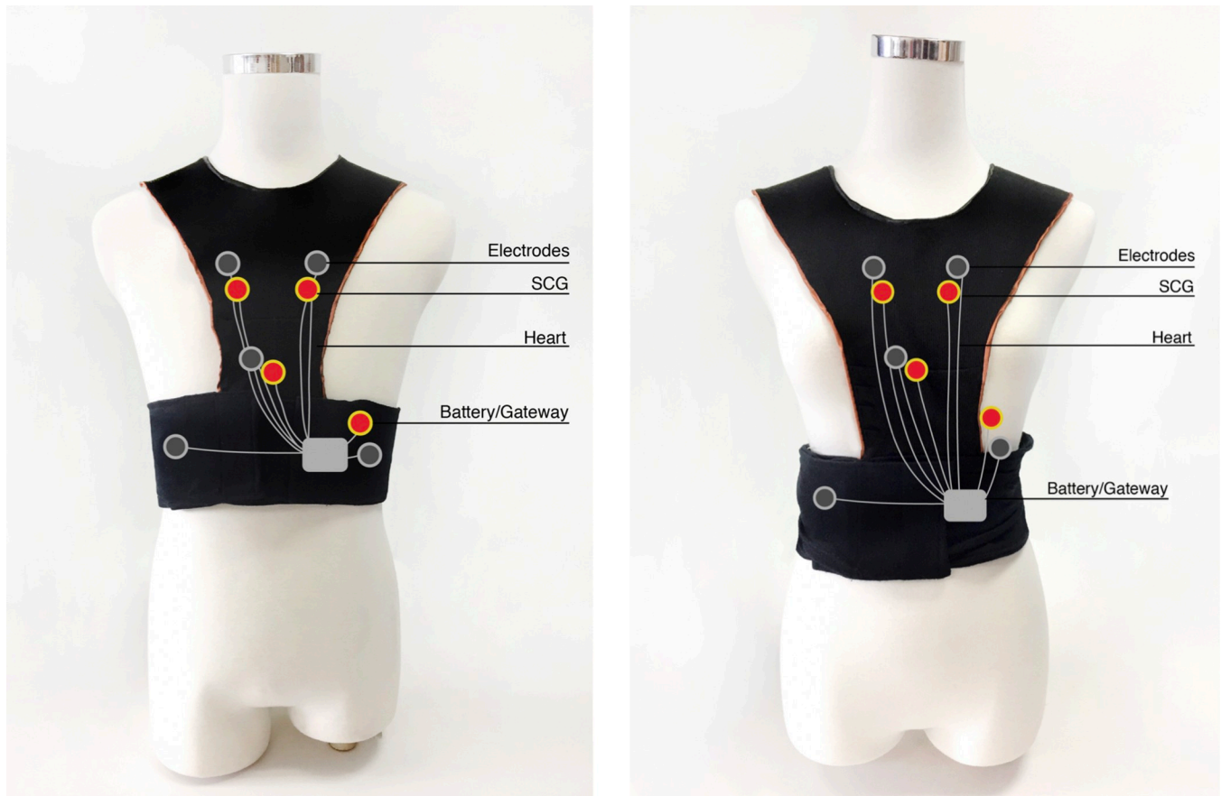
Fig 3. The wearable instrumented vest for males (left) and females (right).
