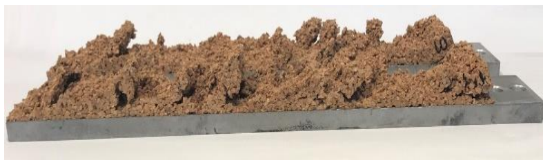
Figure 20. NL10 intergranular fracture after shear test.
