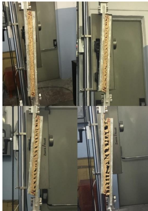
Figure 19. Crack propagation during NL25 shear test.
