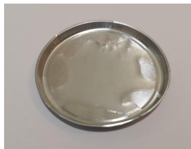
Figure 2. Preparation of epoxy/OMMT thin film for WAXS (Wide-angle X-ray analysis) analysis.
