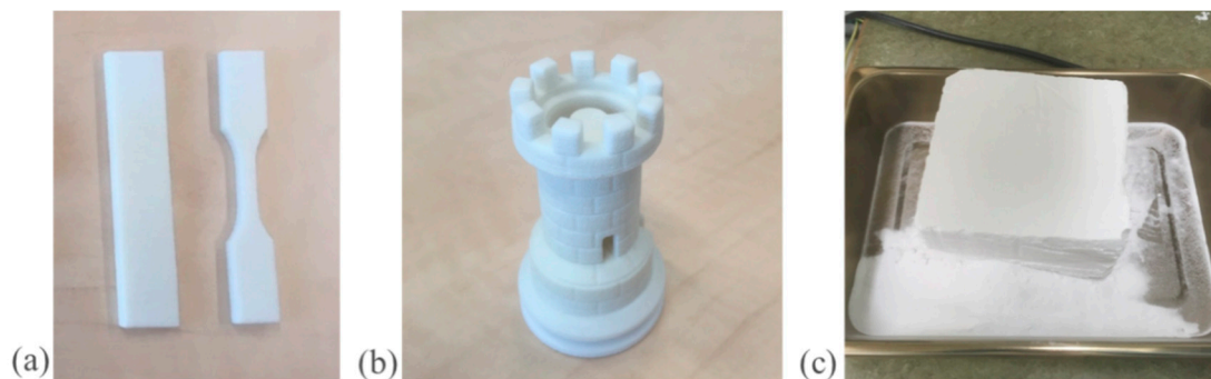
Figure 5. (a) The zx orientation bars printed from PET powder T2. (b) Complex part printed from PET powder T2. (c) The PET powder T2 cake when using the build bed at 228 °C was a little hard.
