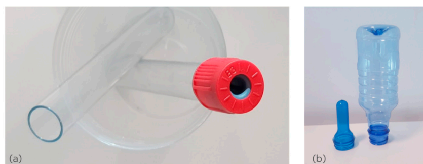
Figure 8. (a) Thin walled injection molded, amorphous PET blood tube. The wall thickness is <1 mm, and hence, the tube is rapidly quenched and is uniformly amorphous. An amorphous PET part like this cannot be made by powder bed fusion. (b) Thin walled injection molded, amorphous PET preforms (left) are converted to semi-crystalline PET articles (biaxially-oriented bottles, right). Amorphous PET parts for post-stretching cannot be made by laser melting of PET powder.
