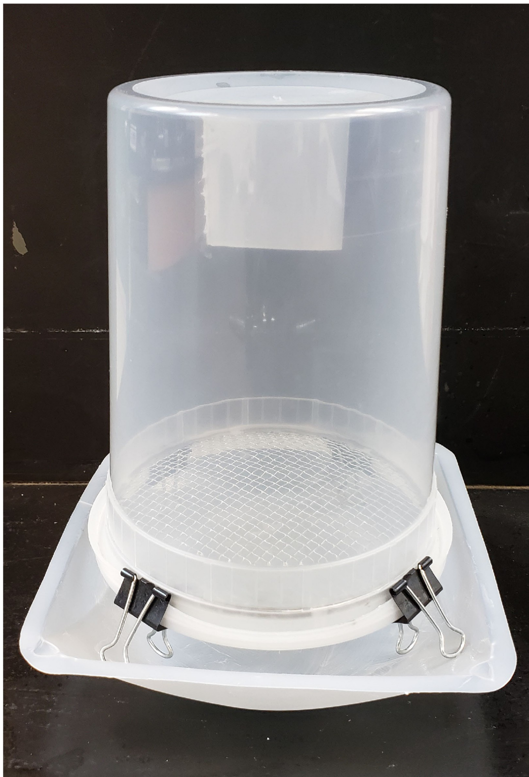
Fig 1. Cage design for Apivar ® efficacy test. A square of Apivar ® was hot glued to the bottom of a plastic container. The screen lid was used to seal the container after bees were added. The container was inverted and suspended over a weighing dish covered in petroleum jelly using binder clips.
