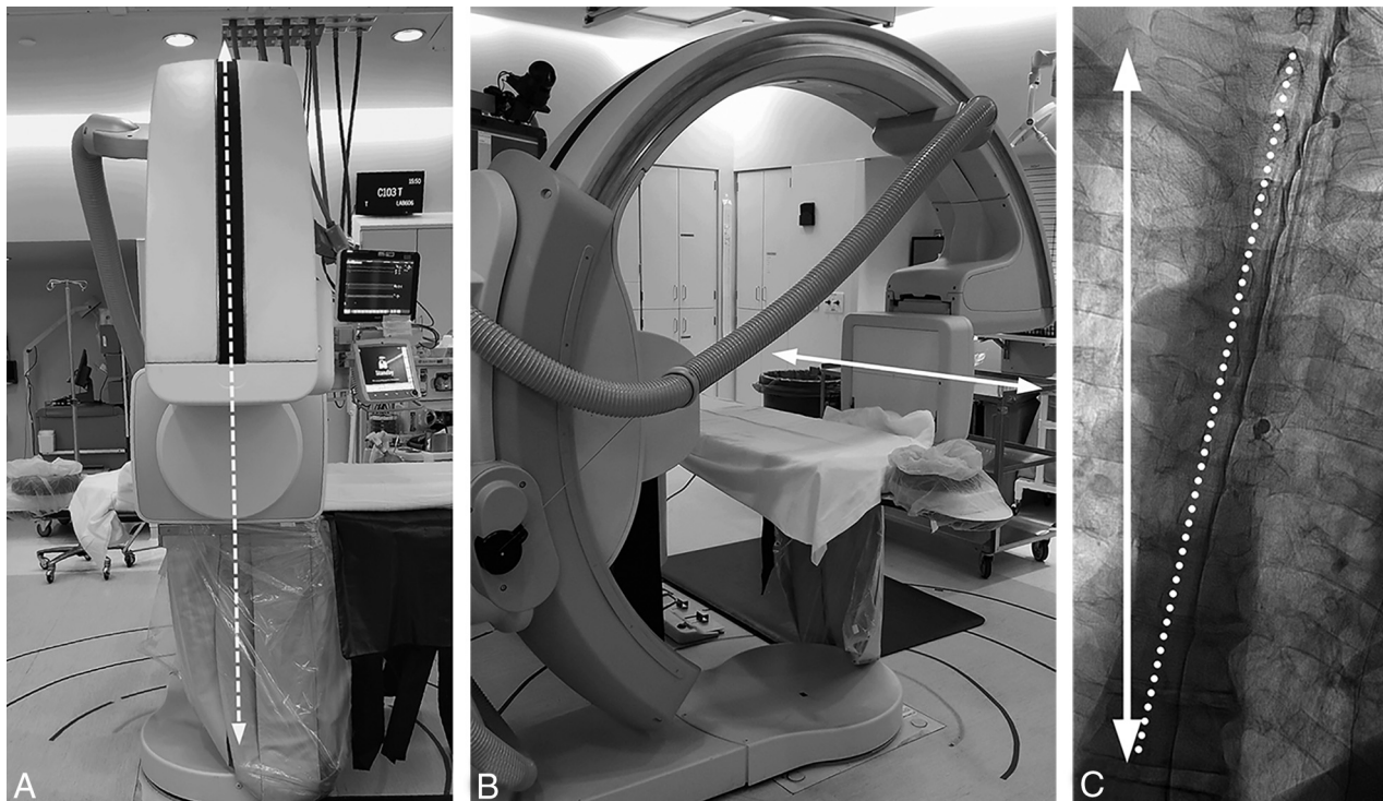
FIG 4. Defining the true horizontal axis and spine tilt on DSM. By placing the C-arm in a vertical position with respect to the floor (A, dotted arrows) while maintaining the long axis of the image intensifier orthogonal to the C-arm (B, solid arrow), the long axis of the image intensifier and the long axis of the image are aligned horizontally, parallel to the floor (B and C, solid arrow). The angle between this line and the line connecting the spinous processes (C, dotted line) defines the spine tilt with respect to the floor.
