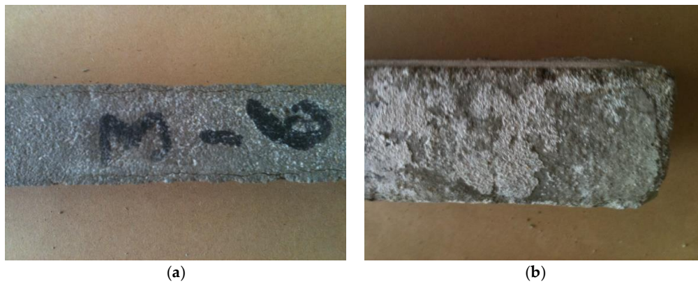
Figure 8. Polymer-cement mortar, p/c = 0.05 , stored in 5% \text{MgSO}_4 solution: (a) after 12 months; (b) after 42 months.
