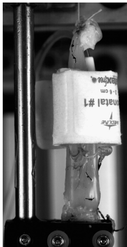
Fig. 1. An isolated bullfrog semimembranosus muscle fit with a small pneumatic pressure cuff. The cuff covers approximately the middle third of the muscle belly. The distal (knee) end of the muscle is connected to a force transducer (above the frame) via Kevlar thread. The proximal (hip) end remains attached to a bony sliver secured in a custom clamp. Small black suture knots allowed tracking of muscle fiber length in high-speed video recordings ( SI Appendix, Fig. S1 ). The muscle pictured is \sim 7 cm in length.
