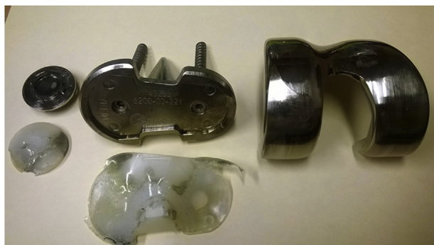
Fig. 6. Retrieved implants showing linear scratches on the femoral component and PE-wear of the metal-backed tibial and patellar components.
