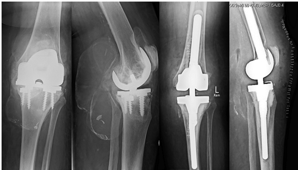
Fig. 1. A case of severe metallosis of the knee joint following fracture of the tibial tray and MoM contact showing the typical radiographic signs (bubble and cloud sign, metal lines and gross metal debris) 20 years after TKA. Revision was done using an RT-Plus system (Smith & Nephew, Memphis, TN).
