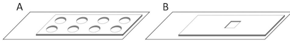
Figure 2: Diagrams of the wells for volume imaging. (A) Diagram of a slide with a silicone isolator. (B) Diagram of a well with multiple layers of tape made by our lab.
