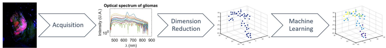
Figure 1. Global view of the proposed machine learning-based prediction of glioma margin by PpIX fluorescence spectroscopic measurements. In this study, the data set is composed of 50 samples from 10 patients. From left to right, the optical spectrum of cells around a tumor is measured. The dimension of the spectral information is then reduced to lower the redundancy. Supervised or unsupervised algorithms are finally used to classify the data and create a prediction of tissue state from the PpIX fluorescence spectroscopic measurements.
