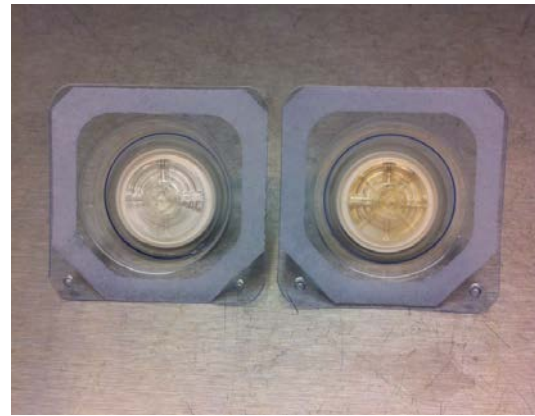
Figure 2 Appearance of filters after filtration of the TPN aq admixture; without addition of trace elements (left) and with \approx 1.5 \text{ mL}/100 \text{ mL} of trace elements (right). A brown colour could be seen on filters that had been in contact with the admixture containing trace elements. The colour disappeared over time.
