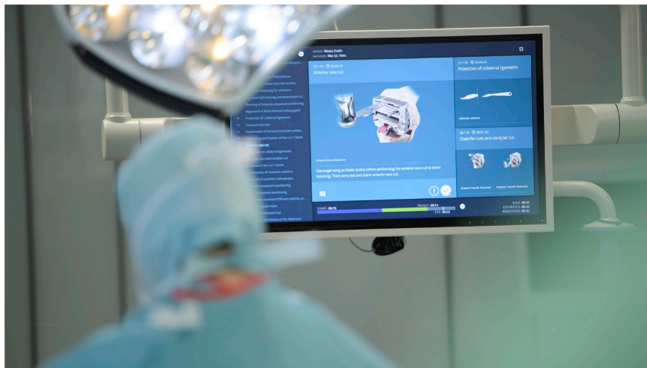
Fig. 3. Intra-OP monitor showing the actual and the next step including the instruments that are required. On the lower part of the screen, the time planning is shown. So a difference between planning and actual time is visualized.
