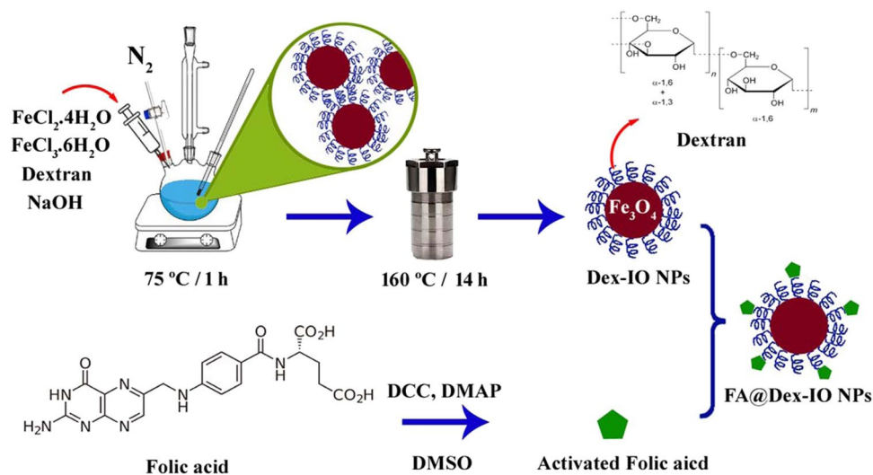
Figure 1. Synthesis process for the preparation of FA@Fe 3 O 4 NPs.
