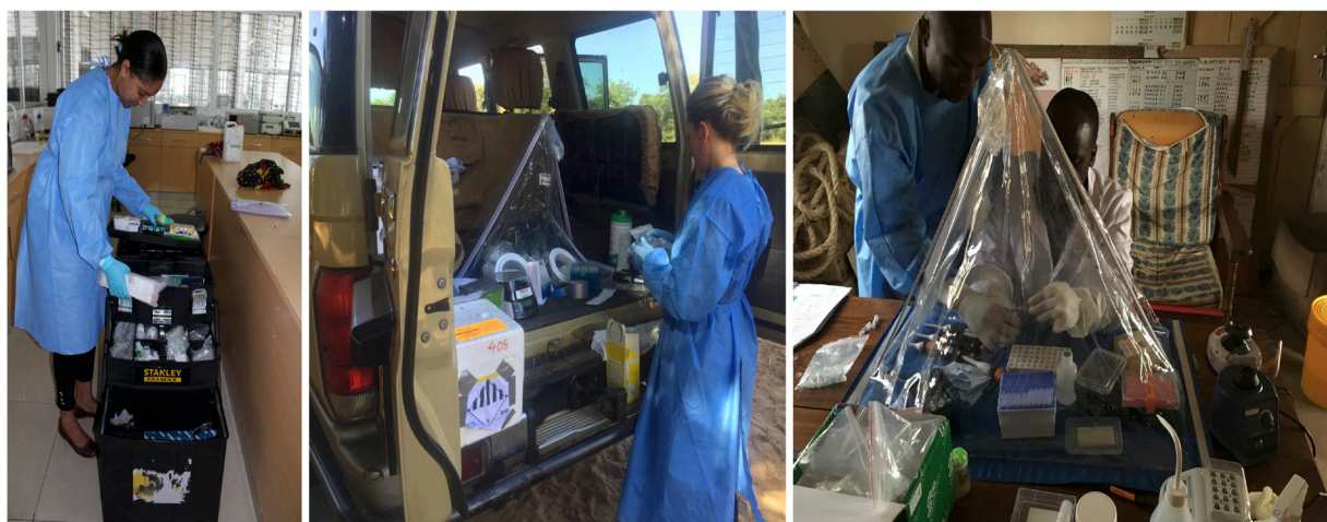
Figure 1. Rabies “lab-in-a-suitcase” setup for sequencing in low-resource settings. A) Lab-in-a-suitcase being used at the Nelson Mandela African Institute of Science and Technology, Tanzania; B) RNA extractions performed in the back of a vehicle using a portable glove box and battery-powered centrifuge in Makueni District, Kenya; C) Laboratory setup for sample inactivations in a district livestock office in Mugumu, Serengeti District, Tanzania.
