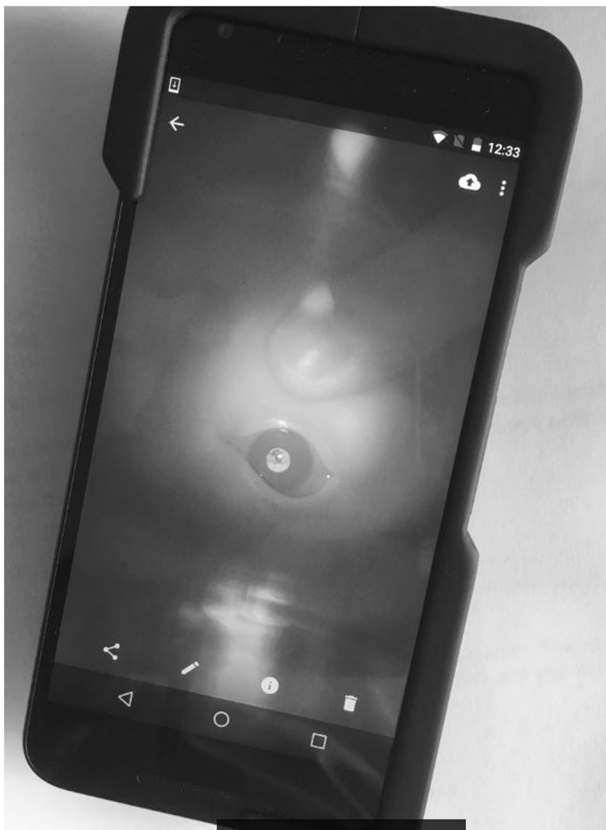
Fig. 1 The modified smartphone IR-reflex imaging camera showing an image of a childhood cataract
