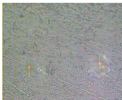
Figure 1. A View of the Effect of the Microhardness Test Indenter on the Enamel.
