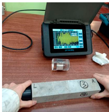
Figure 7. Proceq Pundit 200 ultrasound pulse velocity instrument.
