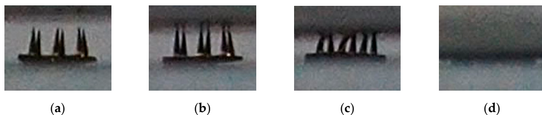
Figure 5. The side face picture of pressing process: (a) before contraction; (b) tip contact the sensor; (c) the needle deformed under the pressure; and (d) the MNs was crushed totally.
