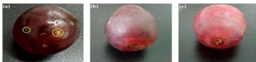
Figure 30. Photographs showing the preservation of red grapes wrapped with (a) plastic film, (b) chitosan film, and (c) chitosan-TiO 2 film at 37 °C for six days. Reproduced with permission from [289]. Copyright Elsevier, 2017.
