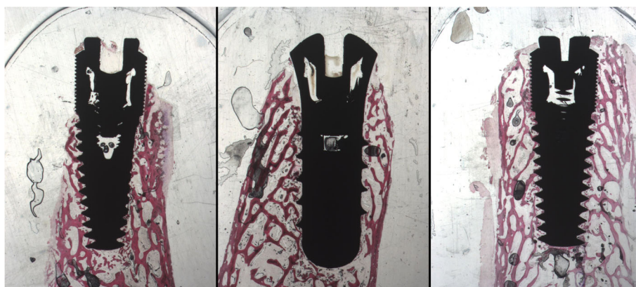
Fig. 5 Optic microscope photo ( \times 9 magnification) after 15 days of implantation. Left side: machined implant (group C). Central photo: sandblasted and acid-etched implant (group A). Right side: laser-treated implant
