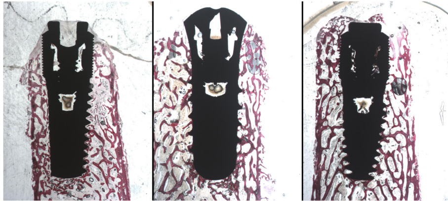
Fig. 6 Optic microscope photo ( \times 9 magnification) after 30 days of implantation. Left side: machined implant (group C). Central photo: sandblasted and acid-etched implant (group A). Right side: laser-treated implant
