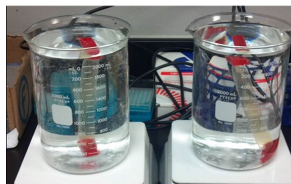
Fig. 2 Purification of succinylated polyethylene glycol (PEG) through dialysis tubing in deionized (DI) water
