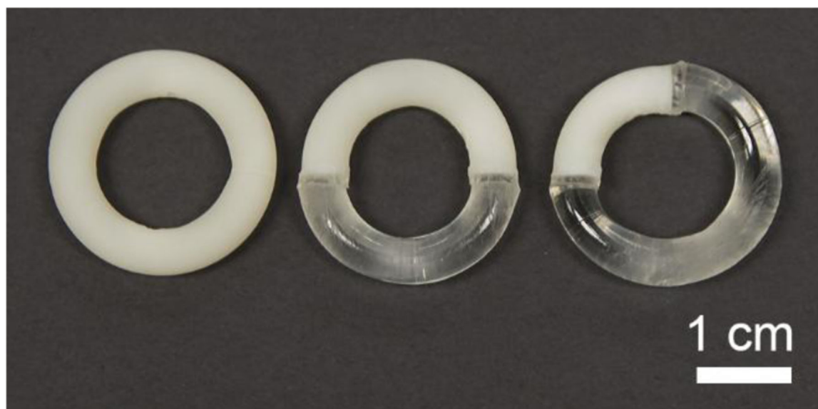
Figure 2. Macaque sized rings containing IQP-0528 were made using injection molding. Drug loaded segment is opaque white. Full rings (left) were made through injection molding. Half (middle) and quarter rings (right) were made by butt-welding a drug loaded segment to an appropriate unloaded segment, as illustrated above.
