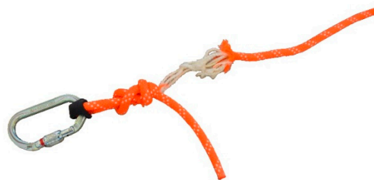
Figure 9. Failure of specimen in Test 10.
