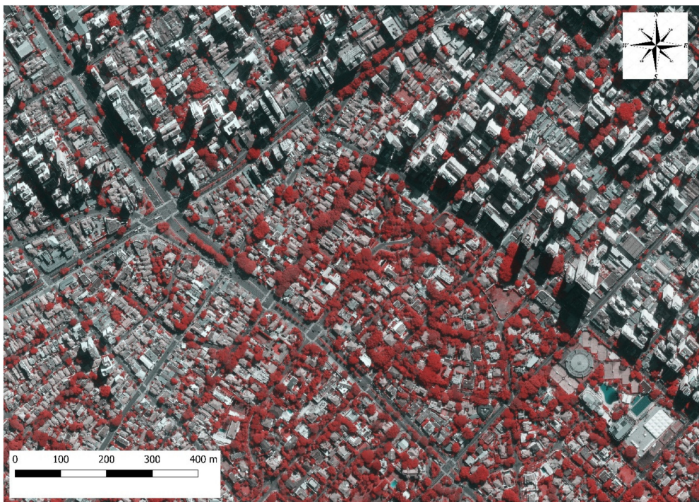
Figure 2. Sample of the orthophoto (2-m spatial resolution) of São Paulo with the near infrared band of QGIS2.18.11, showing green areas in shades of red.
