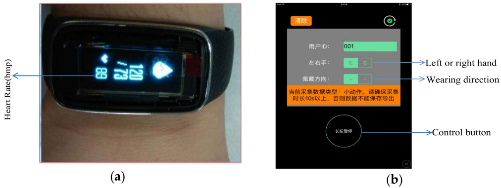
Figure 2. Experimental setup: The heart rate signal of the subject was collected using a smart bracelet (Algoband F8), and the sampling rate of the bracelet was 25 Hz: (a) The bracelet was worn on the subject’s wrist; (b) Connection and data recording APP via Bluetooth.
