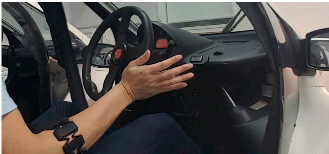
Figure 1. Myo armband used on right forearm to control steering wheel of COMS automobile.
