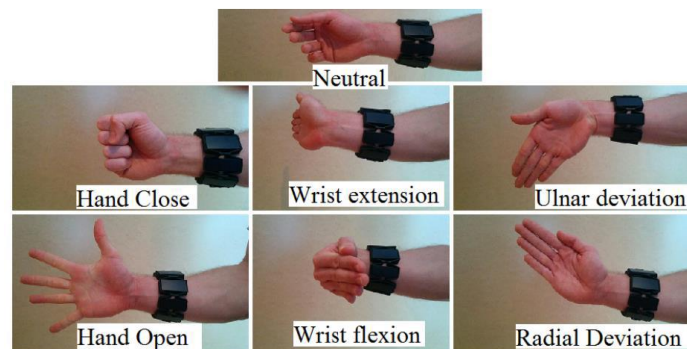
Figure 7. The 7 hand/wrist gestures in the Myo Dataset. In the Myo dataset, seven gestures are included: Neutral, Hand Close, Wrist Extension, Ulnar Deviation, Hand Open, Wrist Flexion, and Radial Deviation.
