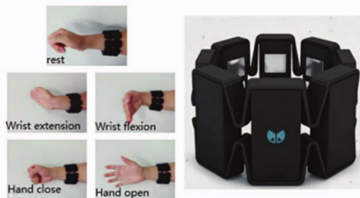
Figure 4. The 5 hand/wrist gestures and Myo armband. In this figure, the left is a schematic diagram of five gestures, and the right is the Myo armband.
