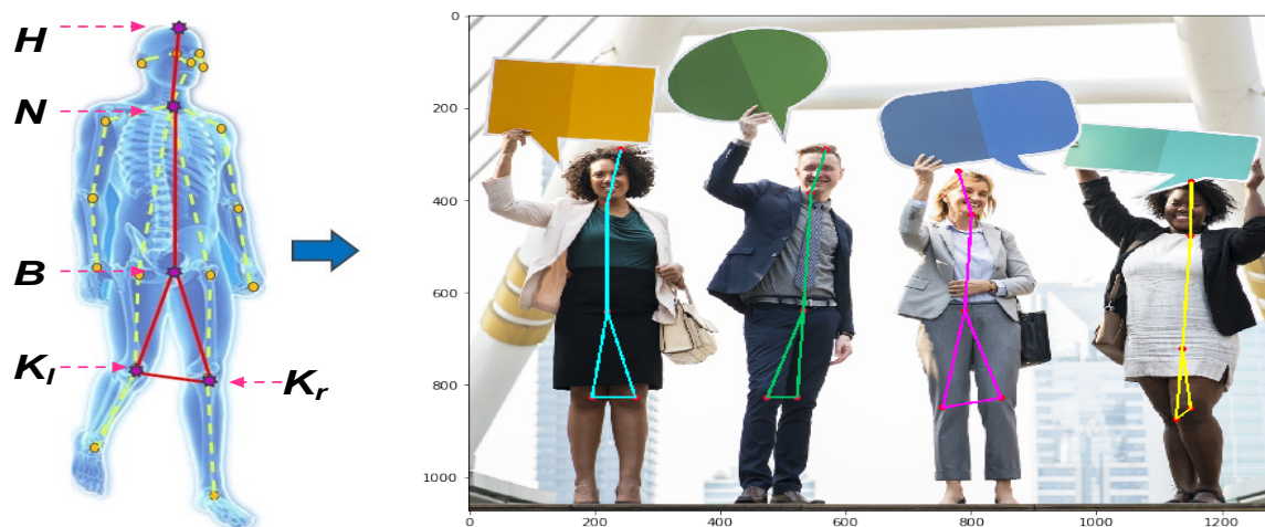
Figure 2. Five-point inverted pendulum model. The left model indicates COCO model [2] that includes 18 key parts of orange color and the yellow dotted line for human skeleton and five-point inverted pendulum model that includes five purple stars and the red real line for human skeleton. In the test, different moving objects (or different persons) indicated by a five-point inverted pendulum model are shown with different colors.
