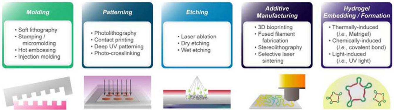
Figure 2. Example manufacturing categories and techniques for microphysiological systems.
