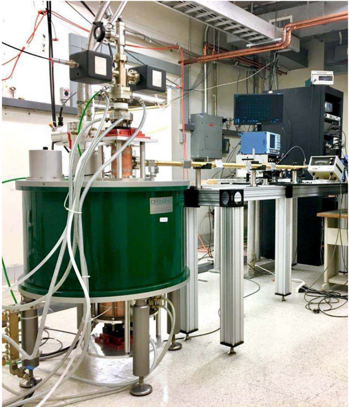
Fig. 6. Photograph of the 527 GHz gyrotron tube under test. A 10 T cryo-free superconducting magnet (green color) is seen in the picture along with the gyrotron tube and a small magnet coil, at the bottom of the main magnet, for fine tuning the electron beam parameters. A 16 mm i.d. corrugated waveguide transmission line made of brass is also seen in the picture.
