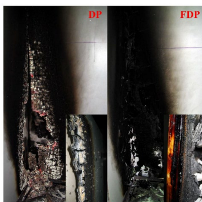
Figure 8. Images from the SBI test of plywood samples.
