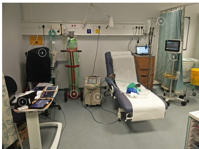
Figure 2 Hypoxia study day set-up. Legend: 1: tablets linked with AMD devices (4 Samsung TAB A, each linked with one AMD: AP-20, WristOX2 3150 BLE, CheckMe™ O2 and VitalPatch®. 1 iPad four connected to the wavelet). 2: resuscitation trolley and oxygen. 3%–7% oxygen in nitrogen cylinder. 4: hypoxicator apparatus. 5: Philips monitor (model MX450) connected to laptop (IX trend software). 6: drip stand with the arterial line pressure bag.
