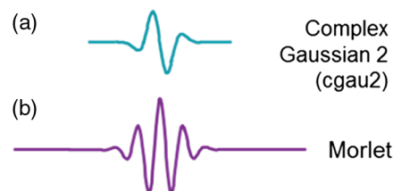
Fig. 2 The waveforms of both wave functions: (a) complex Gaussian 2 (cgau2) and (b) Morlet (bottom).
