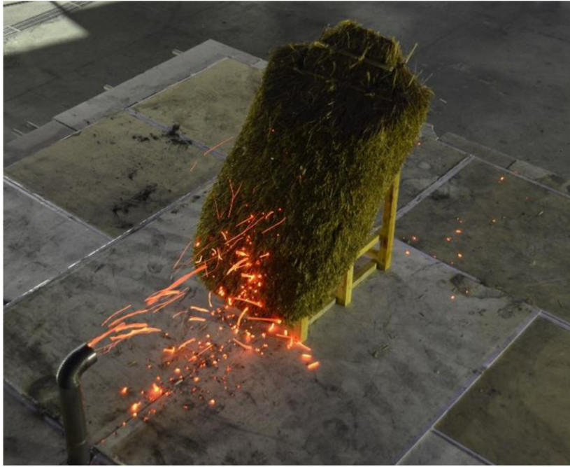
Fig. 12. Thatched roofing assembly (mock-up) exposed to wind-driven firebrand showers characteristic to those generated from structure combustion [132].
